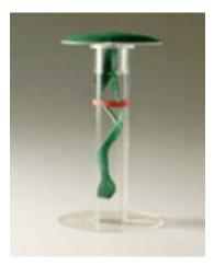
Such level of instrumentation may not fall readily into place in a traditional farm but we developed a very simple evaporation meter which gave a pretty good indication of when to irrigate. The reality is that most farmers have a pretty good eye for their crops and know when to irrigate.
