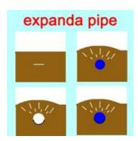
Another idea was the 'expanda' pipe, again with the same objective of getting a mix of air and water into the soil. We ploughed a layflat pipe into the ground, pumped this with high pressure water so the pipe would expand and crack the soil. We then drained the pipe and pumped water into the soil tube left around the pipe directly into the earth.
