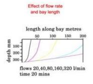
The simulation showed that by using short runs and rapid flows it possible to achieve very high efficiencies and so a system called Micro flood was developed.
