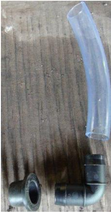
The drain tube is made from fitting readily available from hardware stores. The easiest way to make the hole is to heat up a metal pipe; I use a bit from my socket set, and just melt the plastic. This is much stronger and quicker than drilling which can crack the plastic.
